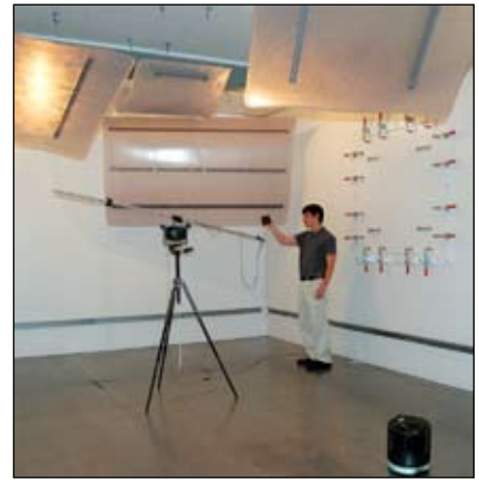
Adam Clark BSME/Acs '12 calibrating a diffuse field microphone on a rotating boom. Transmission Loss pass-through hatch and fixed diffusors are visible behind the student.
